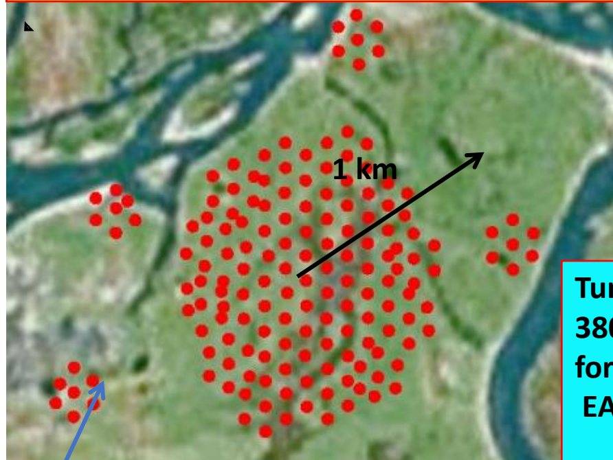
Tunka-133 - 175 optical detectors on the area of 3 km 2
